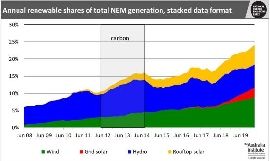
The steady growth of "new" renewable generation (wind and solar) is shown in Figure 4. For the year ending February 2020, grid renewables, i.e. excluding rooftop solar, supplied 19.7% of all generation supplying the NEM grid. When rooftop solar is included, the renewable share increases to 24.3% of all generation, including rooftop solar, in the NEM grid, as seen in Figure 4.
