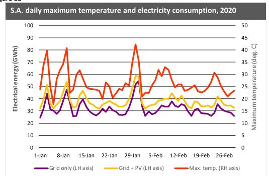
In both graphs the relationship between electricity consumption and maximum temperature is consistently very close. The difference between electricity consumption in 2019 and 2020 is shown in Figure 13. It is obvious that considerably more electricity was consumed in 2019 than in 2020, corresponding to the significantly higher average daily maximum temperatures.
