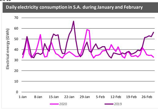
The relationship between hot weather and electricity consumption is of course very well established and understood, both within the electricity supply industry and by anyone interested in energy use in buildings. What makes the relationship so striking, and so important, in South Australia is the combination of several factors, particularly a smaller share of industrial demand for electricity than in other Australian states and
