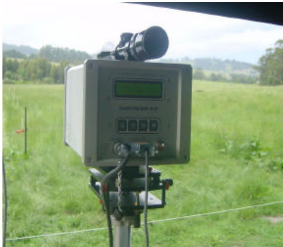
Open path laser measurement of greenhouse gases.
